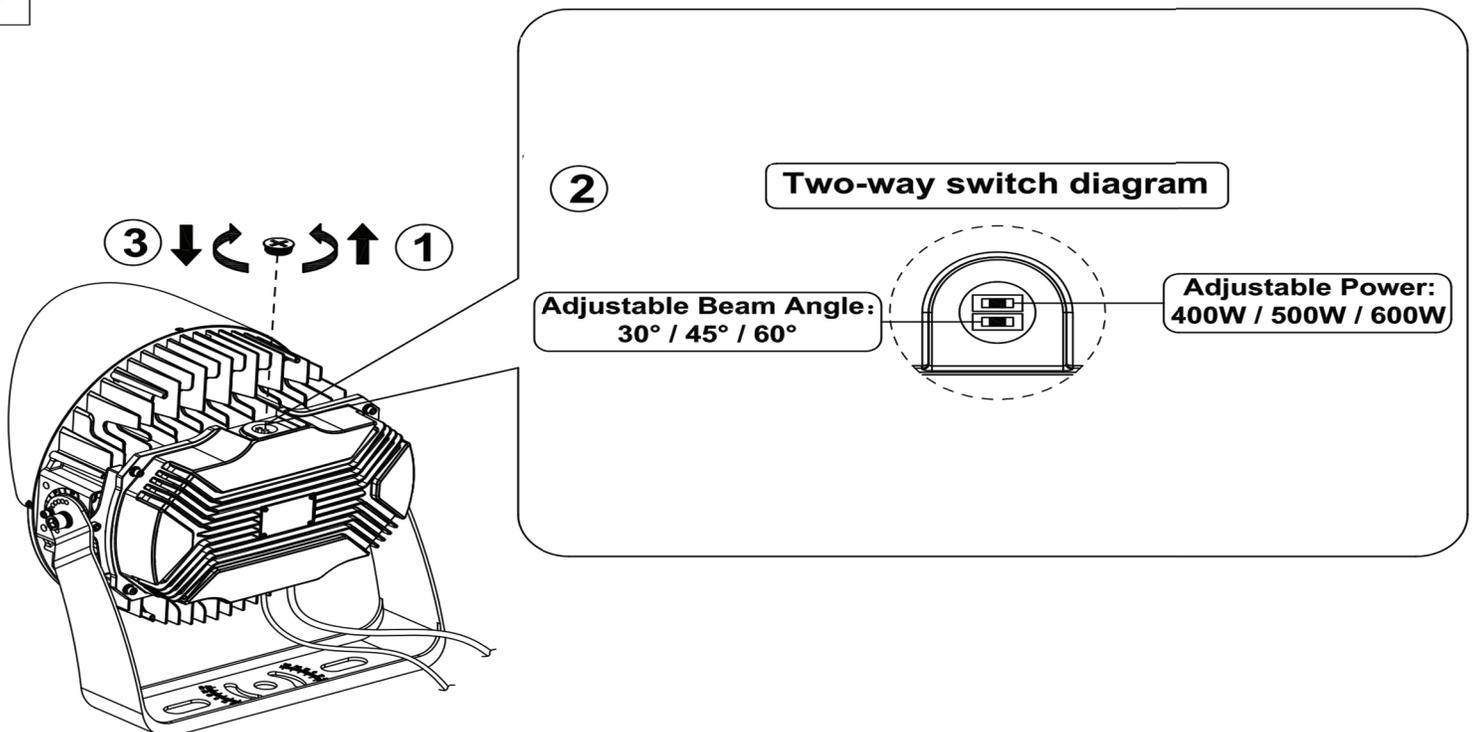
Use a screwdriver to loosen the switch cover. Adjust the light's power and beam angle as needed. After adjustment, reinstall the switch cover and tighten it with a screwdriver. **(Note: All adjustments must be performed with the power off. Live operation is strictly prohibited.)**
