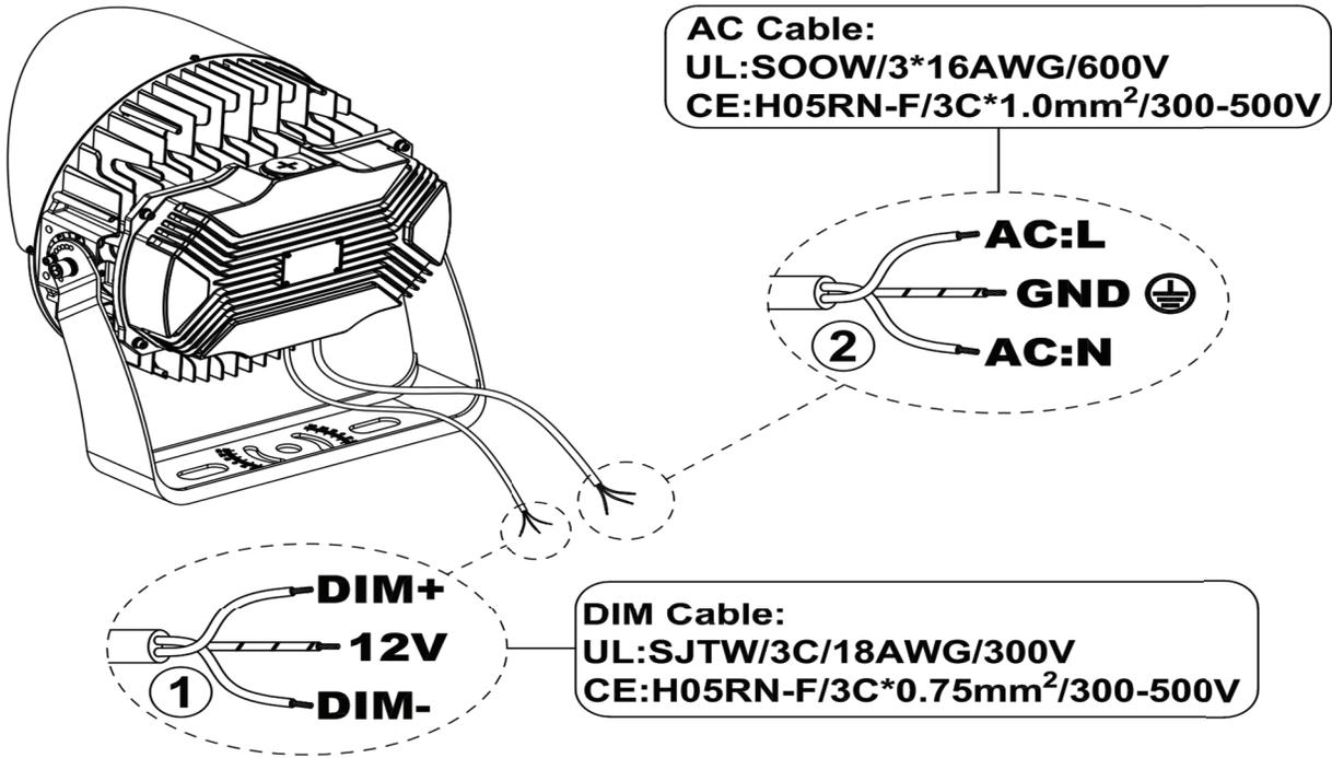
Make all necessary wiring and observe the correct voltage and polarity. Make sure that the electric lines are seated correctly and clamped.
