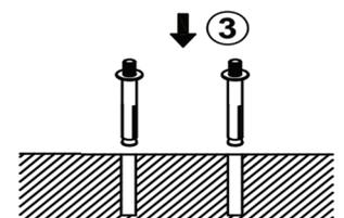
Drill holes at the marked points with a 25mm diameter electric drill bit. Insert the M20 explosive bolt into the hole.
