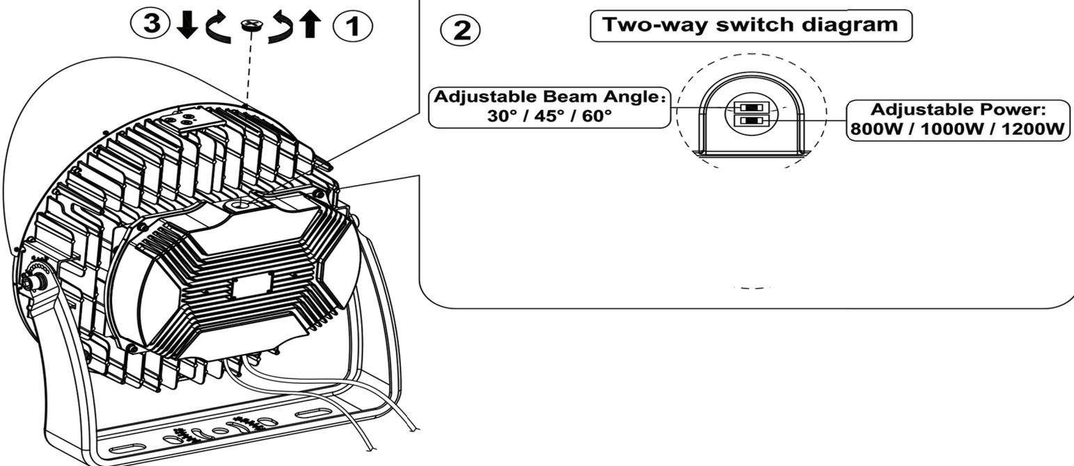
Use a screwdriver to loosen the switch cover. Adjust the light's power and beam angle as needed. After adjustment, reinstall the switch cover and tighten it with a screwdriver. **(Note: All adjustments must be performed with the power off. Live operation is strictly prohibited.)**
