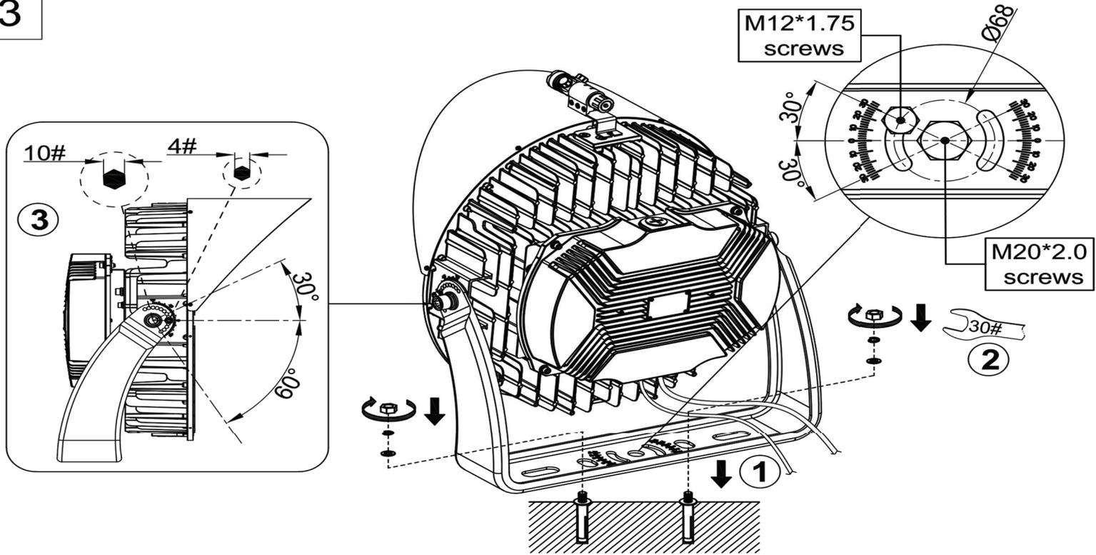
Secure the lamp body to the mounting bracket or mounting surface with the M20 nut and lock the nut. You can use 14 # and 5 # hexagonal spanner to loosen the screws at both ends, adjust the light body irradiation angle (0 ~ 30 degrees and 0 ~ -60 degrees). Secure the middle arc-shaped hole of the bracket with two M12 bolts, allowing the lamp body angle to be adjusted left and right by 30 degrees on each side.
