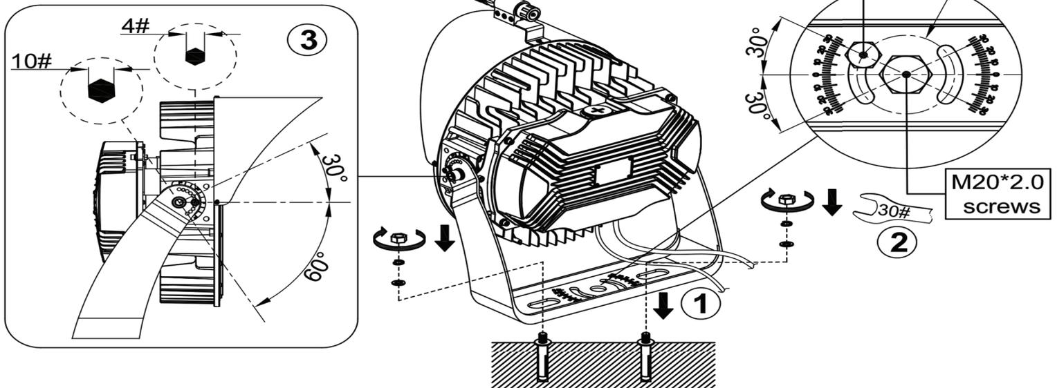
Secure the lamp body to the mounting bracket or mounting surface with the M20 nut and lock the nut. You can use 10 # and 4 # hexagonal spanner to loosen the screws at both ends, adjust the light body irradiation angle (0 ~ 30 degrees and 0 ~ -60 degrees). Secure the middle arc-shaped hole of the bracket with two M12 bolts, allowing the lamp body angle to be adjusted left and right by 30 degrees on each side.
