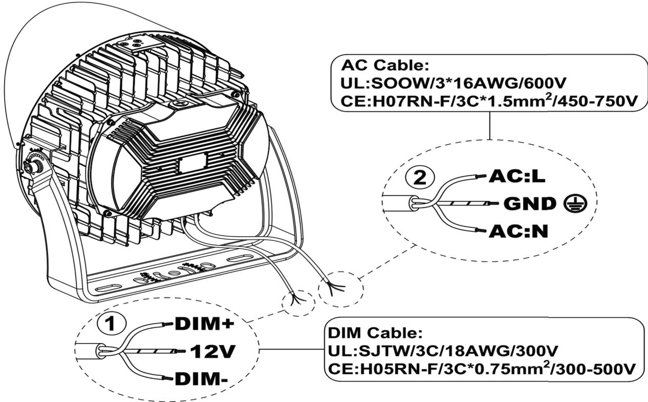
Make all necessary wiring and observe the correct voltage and polarity. Make sure that the electric lines are seated correctly and clamped.
