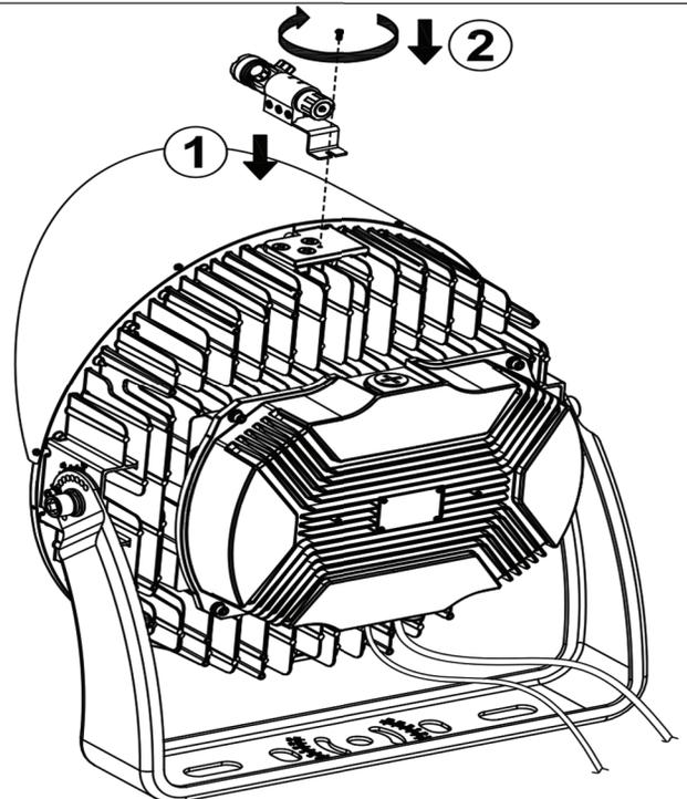
Take the Visor from the box, align the mounting holes with the luminaire. Take the Screw, fit visor.
