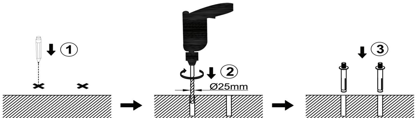
Drill holes at the marked points with a 25mm diameter electric drill bit.
