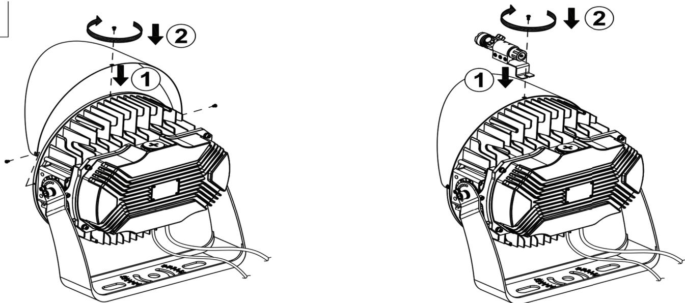
Take the Visor from the box, align the mounting holes with the luminaire.
