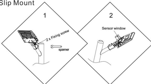
Slip fitter mounts are very easy to install as they usually slide over standard 2 3/8-inch lighting poles.
