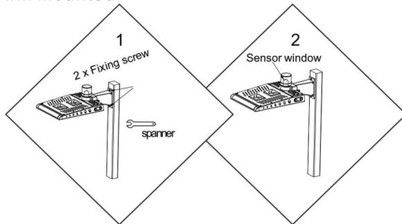
Drill holes on the square pole corresponding to the holes on the arm, and use the bolt and nut plate to fix the fixture to the pole tightly.
