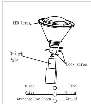
1. Connect the AC wire of the lamp as shown in the picture, then insert the lamp into the 3-inch pole.
