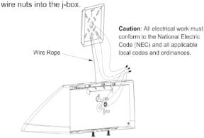
Stick EVA gaskets on the back of the wall mounting plate properly, which is very important for water proof. Fix the wall mounting plate on the junction box according to the arrow pointing upwards. Note that the wall mounting plate must be leveled before tightening the screws.
