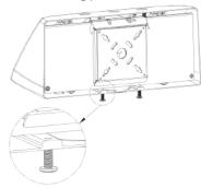
3. Hang the fixture on the wall mounting plate with a wire rope, and pay attention to protect the surface of the fixture during installation to prevent scratches and damage to the surface. Ensure the line voltage at the fixture is correct, make all necessary wiring connections, and push all the wires and wire puts into the i-box.
