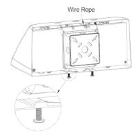
Note: To ensure waterproof seal, apply weatherproof silicone sealant around out edge of fixture (For mounting box installation, apply silicone around the edge of mounting box ), make sure to fill the gap between fixture and wall.
