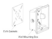
3. Hang the fixture on the wall mounting box with a wire rope, and pay attention to protect the surface of the fixture during installation to prevent scratches and damage to the surface. Ensure the line voltage at the fixture is correct, make all necessary wiring connections, and push all the wires and wire nuts into the j-box.
