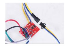
If lamp does not light as the above: Take apart the lamp cover Check circuit, if connector is dropping out, light on, then install.
