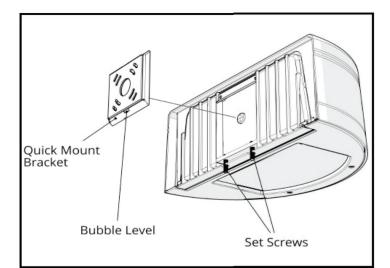
**Step 2:** Remove the quick mount bracket from the fixture and attach it to the junction box with the appropriate hardware (not included).
