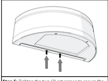
**Step 5:** Tighten the two (2) set screws to secure the fixture housing to the quick mount bracket.
