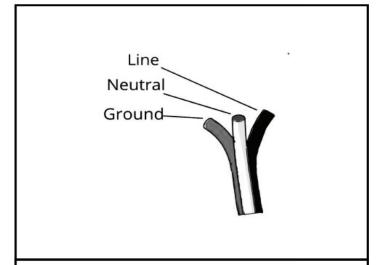
**Step 3:** Make the wiring connections according to the wiring diagram on Page 4. Push excess wire into the junction box.
