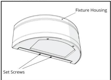
**Step 1:** Loosen the two (2) set screws found on the bottom of the fixture housing.
