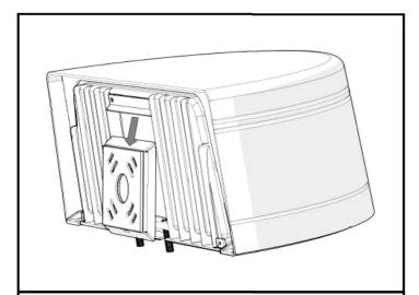
**Step 4:** Lift the fixture and tilt slightly toward the quick mount bracket. Hook the fixture housing onto the quick mount bracket as shown. Take care not to pinch any wires.
