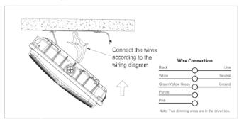
2. Fix the mounting plate to the ceiling with the screws.
