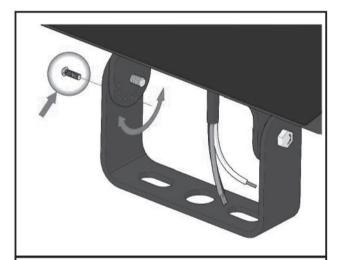
**Step 3:** To aim the fixture, use a screwdriver to loosen the machine screw. Move the fixture head to the appropriate position and tighten the screw in one of the threaded slots to lock it in position.
