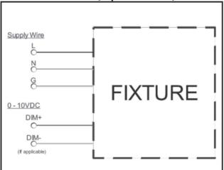
**Step 1:** Make the wiring connections according to the diagram on Page 6. If dimming is not required, make sure the dimming leads are capped.
