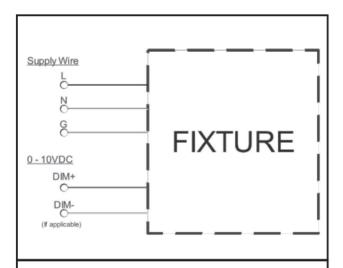
**Step 2:** Make the wiring connections according to the diagram on Page 6. If dimming is not required, make sure the dimming leads are capped.
