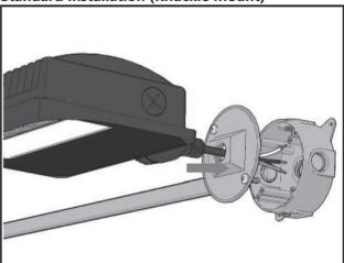
**Step 1:** Feed the power cord into the junction box or conduit. If j-box mounted, insert the threaded portion of the knuckle into the desired knock-out on the junction box.
