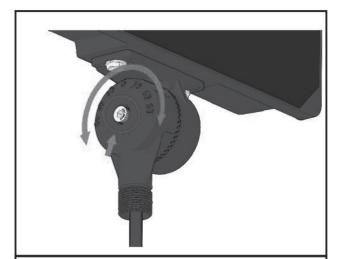
**Step 3:** To aim the fixture, use a hex key to loosen the machine screw. Move the fixture head to the appropriate position and tighten the screw to lock it in position.
