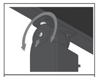
**Step 3:** To aim the fixture, use a hex key to loosen the machine screw on the slipfitter. Move the fixture head to the appropriate position and tighten the screw to lock it in position.
