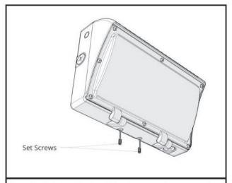
**Step 5:** Tighten the two (2) set screws to secure the fixture housing to the quick mount bracket.
