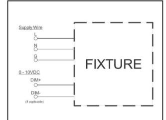
**Step 3:** Make the wiring connections according to the wiring diagrams on Page 4. Push excess wire into the junction box.
