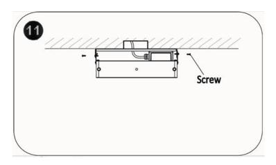
**STEP 4:** Push the hook on the other side of lightbody to the mounting bracket, and fix lightbody to mounting bracket using locking screws to complete installation (see Figure 11).
