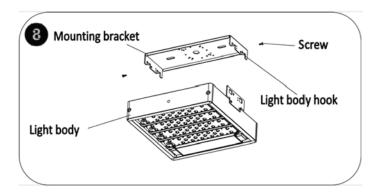
**STEP 1:** Remove mounting bracket from lightbody by loosening the screws on both sides of the brackets (**See Figure 8**).
