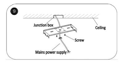
**STEP 2:** Get mains power supply cord through wiring hole on the mounting bracket, and fix the mounting bracket to ceiling or the junction box in ceiling using swelling bolt or screw.(**See figure 9**)
