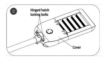
**STEP 3:** Loosen hinged hatch locking bolts with 5mm hex wrench or its equivalent, and open the hatch for led driver compartment access. **See Figure 2.**
