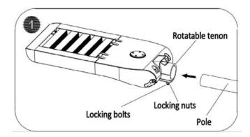
**STEP 1:** Loosen nuts from pole locking bolts, then slide fixture on to pole through opening (tenon) on the rear of housing. **See Figure 1.**
