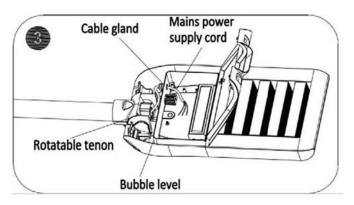
**STEP 4:** Get mains power supply cord into led driver compartment via cable gland, and use open spanner or similar tool to lock the gland to mains power supply cord tightly. **See**
