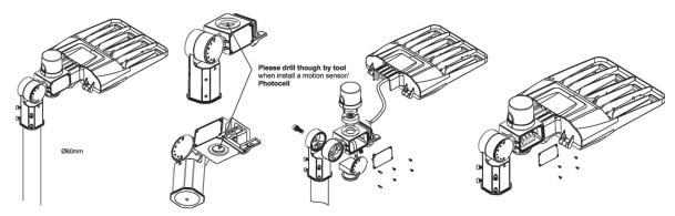
How to install a photocell/ motion sensor on EA/PD bracket
