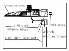
Method 2: install the 3 inch adapter piece on the lamp, then install the 1.6-inch adapter piece on the lamp post, install on the 1.66-inch lamp lever, tighten the two screws, the lamppost is fixed. Lamps of lamps and lanterns can adjust the Angle of lamps and lanterns. (5  $^{\circ}$  / 2.5  $^{\circ}$  0  $^{\circ}$  / 2.5  $^{\circ}$  / - 5  $^{\circ}$  ). (see charts.)
