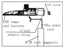
Mode 3: when the lamppost is turned into a lamppost 2.38 inches, the lamp is mounted directly on the lamp, with two screws and the lamppost fixed. The Angle of lamps and lanterns adjusts according to actual situation. Lamps and lanterns (5  $^{\circ}$  / 2.5  $^{\circ}$  Angle 0  $^{\circ}$  / 2.5  $^{\circ}$  / -5  $^{\circ}$  ) (as shown)
