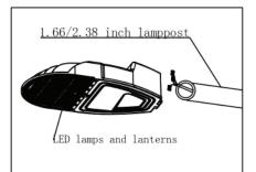
Method 1: the lamps and lanterns directly install the lamp rod, the outer diameter of the lamp pole is 3 inches and 2.4 inches two kinds of specifications. When the street lamp is assembled into the lamp post, the Angle of the lamp will be adjusted according to the actual situation. (5  $^\circ$  for lamps and lanterns with Angle / 2.5  $^\circ$  0  $^\circ$  / 2.5  $^\circ$  / -5  $^\circ$  ) (as shown)
