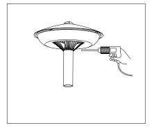
2). Lock the screws on both sides of the lamps, fix the lamps on the pole.
