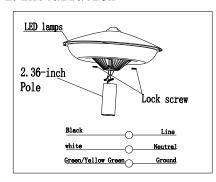
1). Connect the AC wire of the lamp as shown in the picture, then insert the lamp into the 2.36-inch pole.
