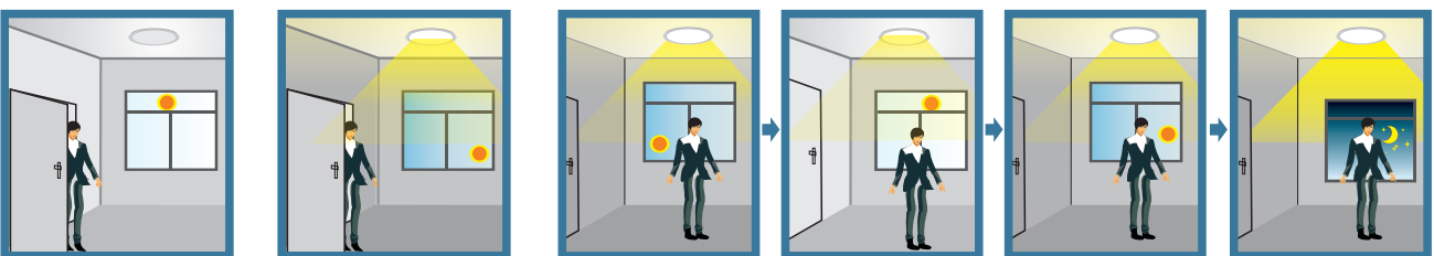
Ambient light larger than preset illumination level (Set by 1-10V daylight sensor), the lamp keeps off.
