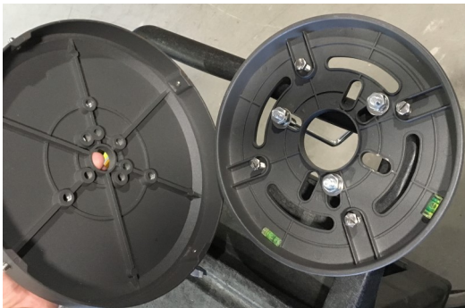
Top plate can be rotated to position Bollard. Top plate is secured to bottom plate with set screws (4).
