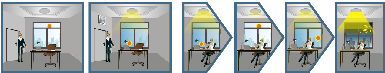
Ambient light larger than preset illumination level (Set by 1-10V daylight sensor), the lamp keeps off.
